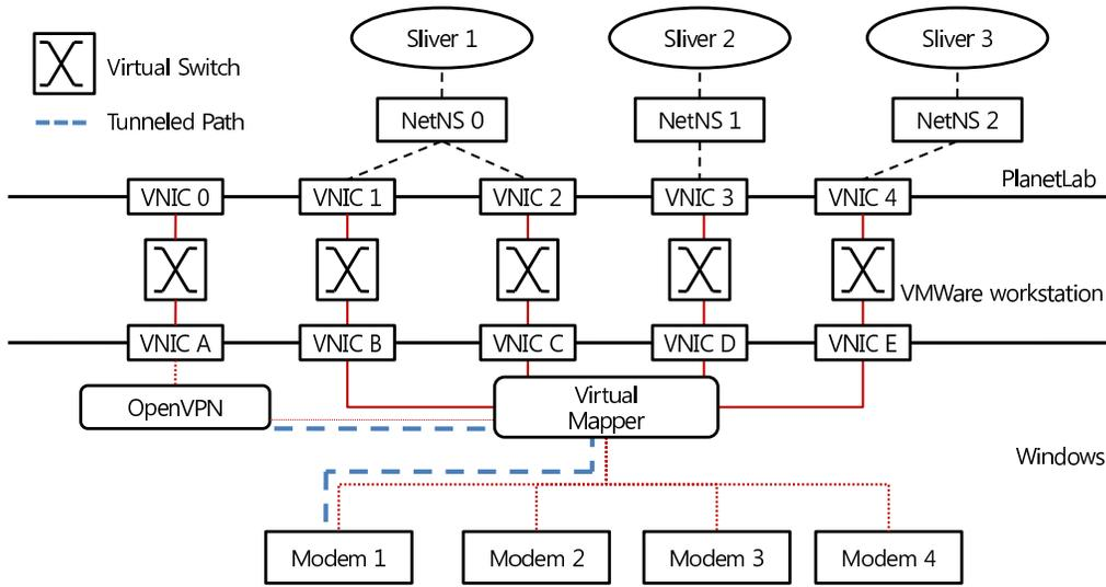
Figure 1: Network subsystem of a mobile PlanetLab node
