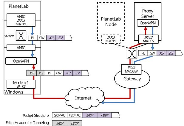
Figure 2: Packet encapsulation and decapsulation through a proxy server
